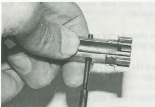
Depress rear of extractor and punch out extractor pin.
