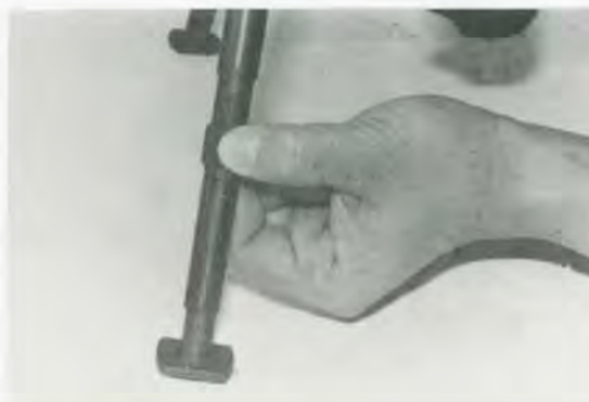
Depress the button and pull downward to extend the leg.
