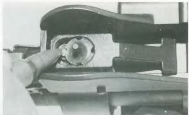
Fig. 2.4. 1a Adjustment of Post Front Sight.
