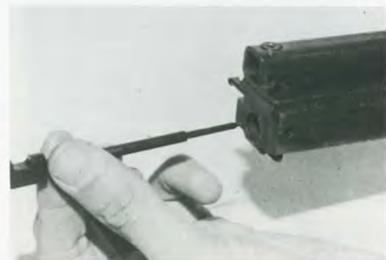
d) Remove firing pin
