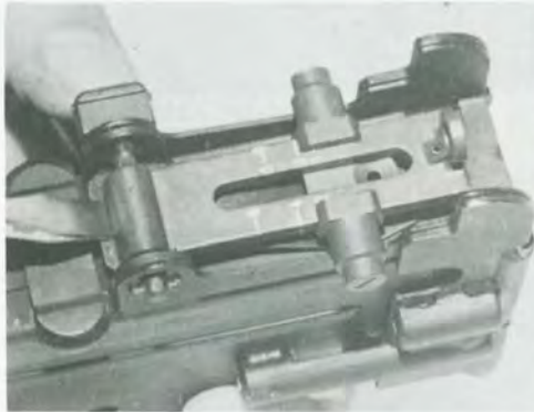
Depress sight leaf spring and windage screw. Remove sight lock pin.
