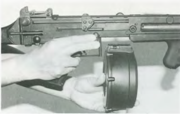
Fig. 2. 1a Remove magazine by depressing the magazine catch on the right hand side of the receiver.
