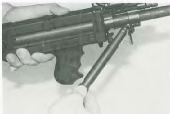
Pull and pivot the bipod leg to unfold the leg.
