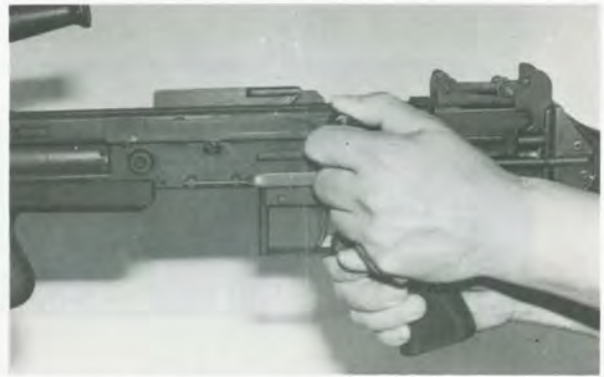
Fig. 2. 1b 1) Cock the weapon by twisting the knob anti-clockwise and pull back fully then return knob to original position. 2) Put selector on 'S' position.
