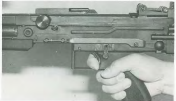
Fig. 2.1d Point the weapon in a safe direction, pull the trigger and put selector back to 'S' position.
